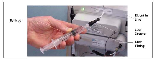
Figure B-22. Assembled Syringe and Luer Adapter
